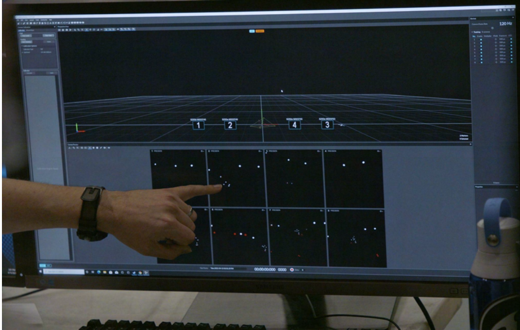
Figure 8: A Motive panel shows each camera's view of the detected markers.
