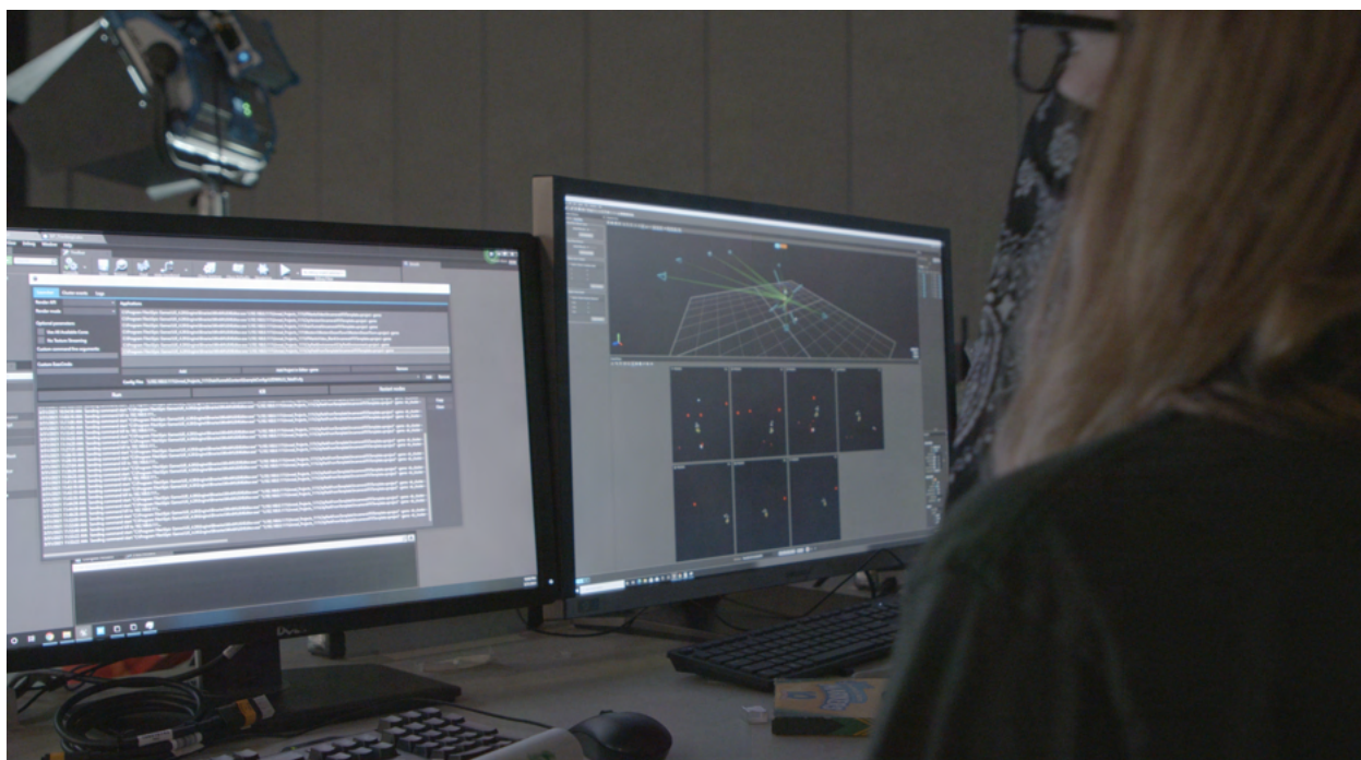
Figure 60: OptiTrack software, Motive, streaming data from a rigid body into Unreal Engine.
