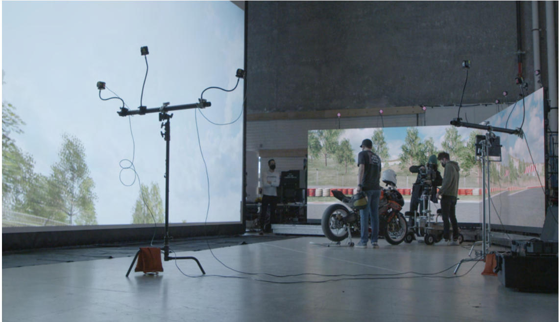
Figure 27: Two renders of the Unreal project simultaneously displayed on both LED walls and the projector using nDisplay.
