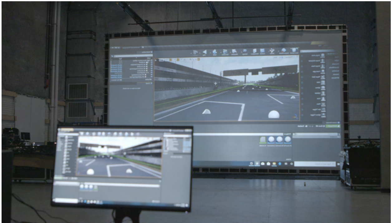
Figure 4: Draper StageScreen displaying an Unreal Engine project driven by a PC.
