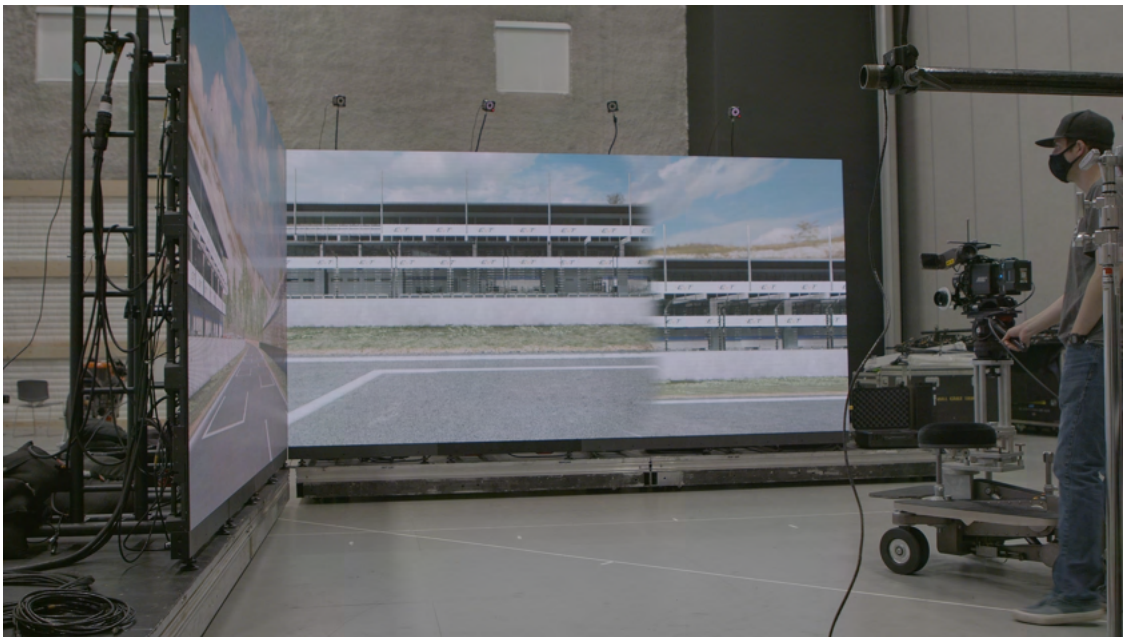
Figure 23: Co-Director testing the inner frustum render with a tracked camera.
