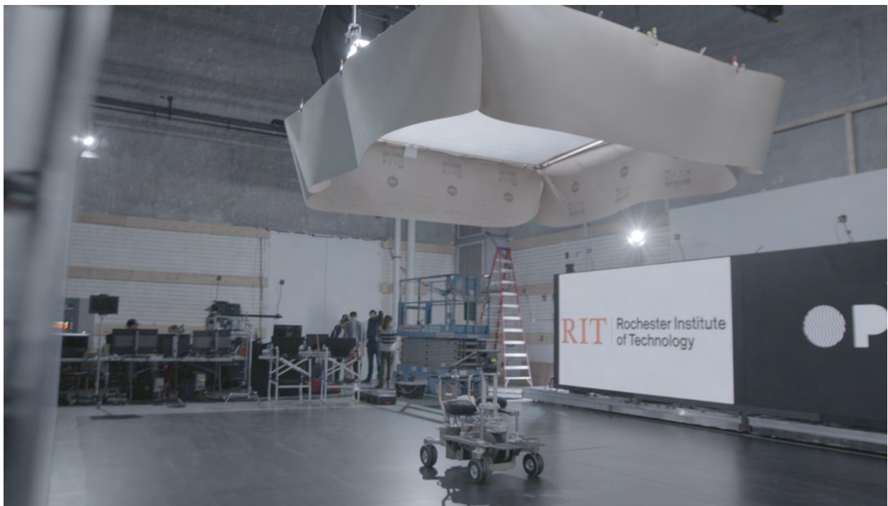
Figure 38: Final lighting setup with additional curtains to direct the lighting onto the center of the set.
