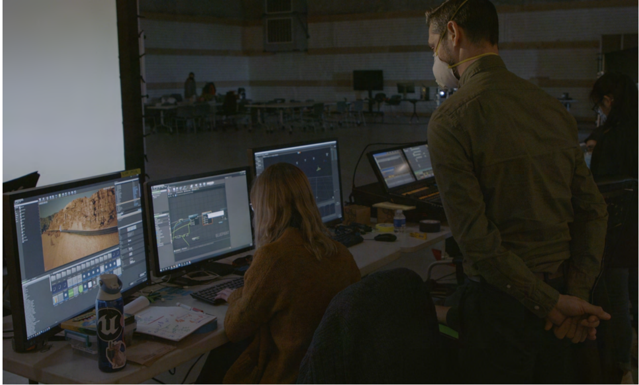
Figure 61: Workstation setup with a PC driving the virtual set in Unreal (left), and another streaming the tracking data from Motive (right).
