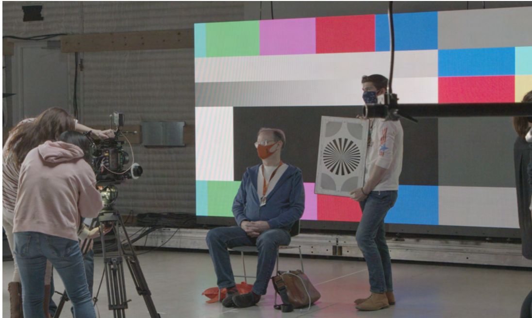
Figure 10: RIT students focusing Arri Alexa Mini on a subject for aliasing analysis with a test background image on the LED walls.
