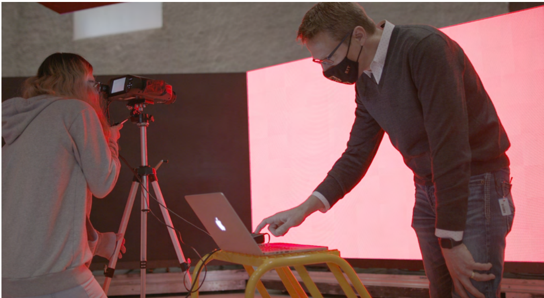
Figure 14: An RIT student and faculty member take colorimetric measurements using the PR655 spectrometer.
