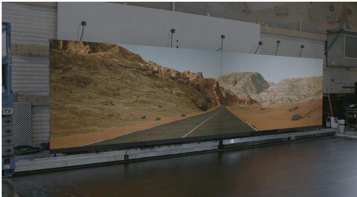
Figure 59: Full LED wall setup with OptiTrack cameras attached to the top.
