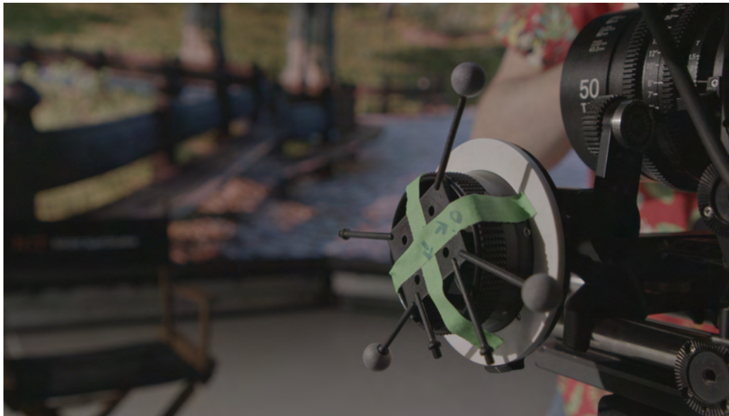
Figure 24: Virtual follow focus rig with OptiTrack markers.
