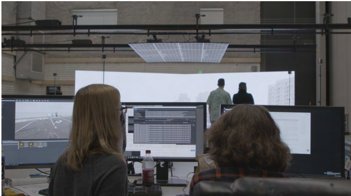
Figure 5: Workstation screen setup with Motive on the right monitor and Unreal Engine and nDisplay on the left and center monitors respectively.
