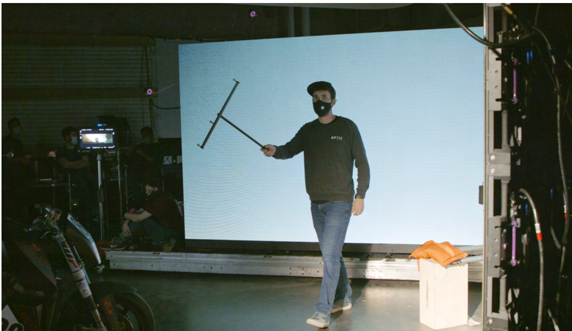
Figure 9: Co-Director performing the wanding process to calibrate the OptiTrack system.
